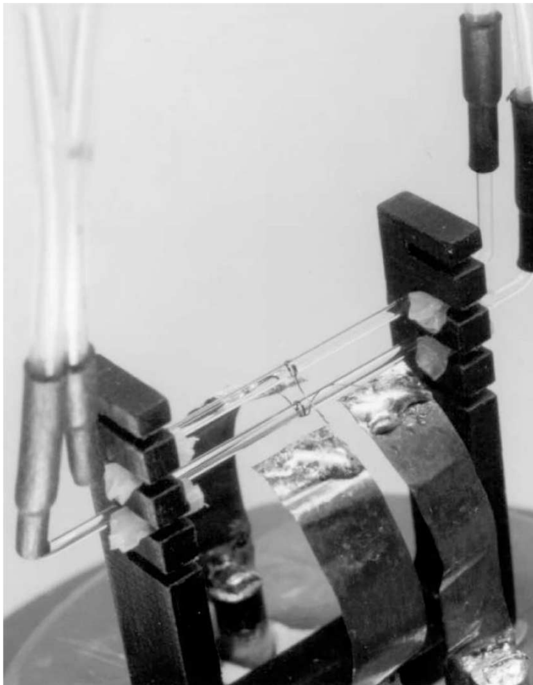
FIG. 2. Photograph of the sample capillaries and coils used in the NMR Difference Probe.
